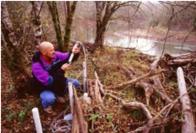
Figure 4.2. To measure nitrogen runoff in the Pacific Northwest, plant physiologist Steve Griffith collects water samples from a monitor well inside the riparian zone near the Calapooya River. Photo by Brian Prechtel, Agricultural Research Service, U.S. Department of Agriculture, Beltsville, Maryland.
